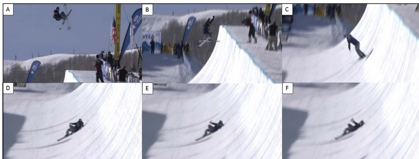
Figure 4 Case 1 (50 Hz). Key crash events: (A) the highest point of the athlete's trajectory, (B) descending towards the vertical part of halfpipe wall, (C) ski landing frame (first impact of ski tails), (D) buttocks and lower back contact with snow, (E) upper back contact with snow, (F) head impact frame.
