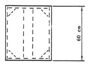
Note: Top and sides are 3/4" plywood. Interior braces are 2"x4".
