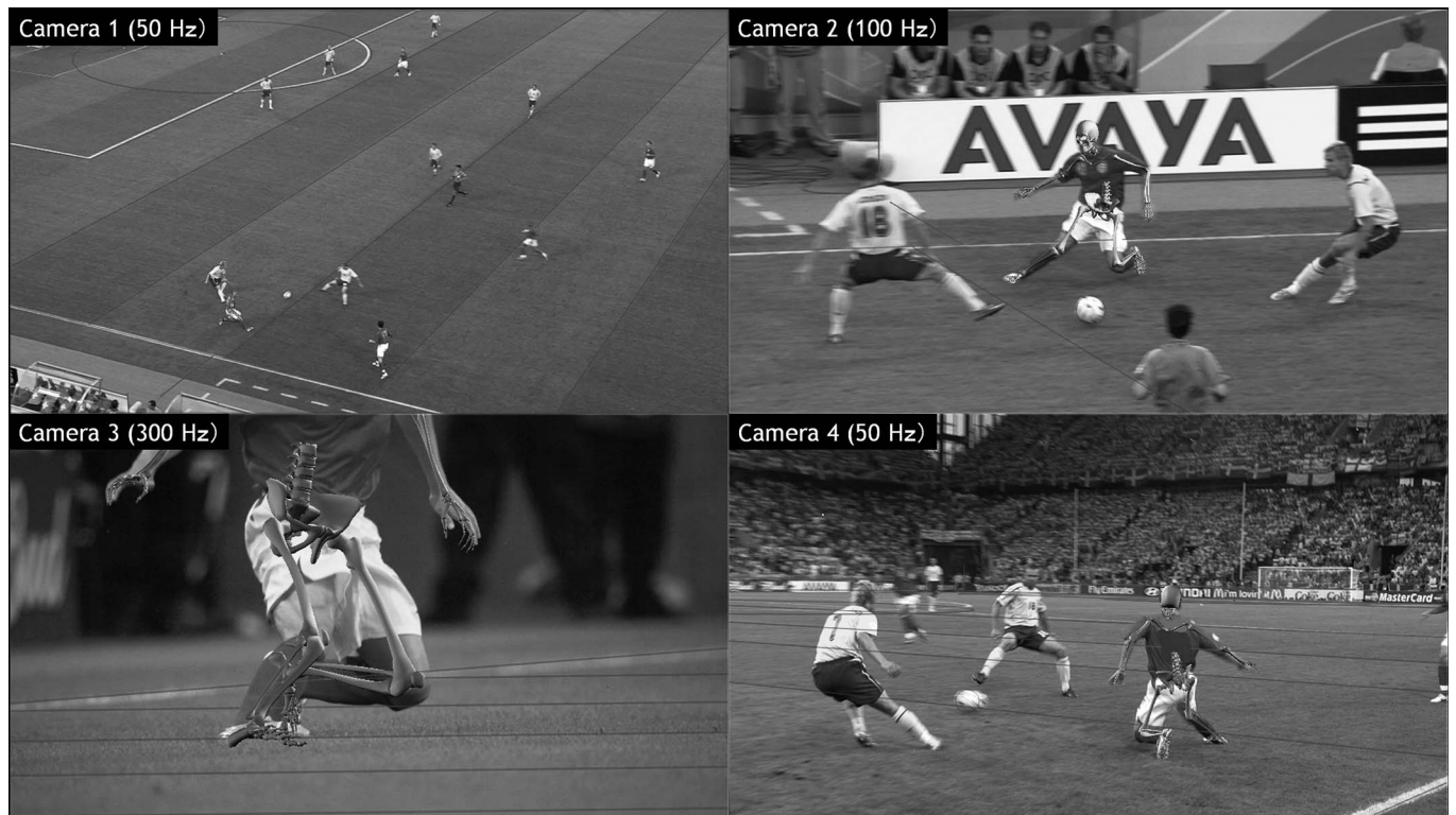
FIGURE 1. A frame of the matched video in Poser. The injury situation 30 milliseconds after IC. Each panel shows the customized skeleton model and the football pitch model superimposed on and matched with the background video image from each camera. Cameras 1 and 4 had an effective frame rate after being deinterlaced of 50 Hz, camera 2 had 100 Hz, and camera 3 had 300 Hz.
